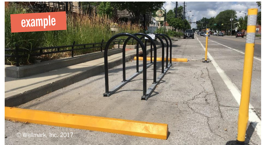
Example of a bike corral, installed in a former on-street parking space. This type of bike parking could work well in downtown Martin.
